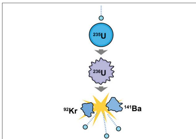
Figure 2: A diagram showing an example of nuclear fission (from [http://en.wikipedia.org/wiki/File:Nuclear\\_fission.svg](http://en.wikipedia.org/wiki/File:Nuclear_fission.svg))
