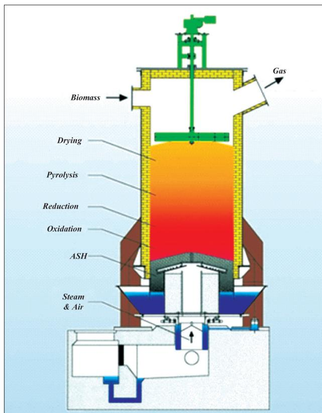
**Figure 3: A gasifier (which converts carbonaceous materials, such as coal, petroleum, biofuel, or biomass, into carbon monoxide and hydrogen) in the process of pyrolyzation (from [http://www.worldchanging.com/gasifier\\_zones.jpg](http://www.worldchanging.com/gasifier_zones.jpg))**
