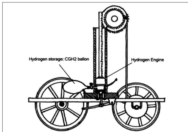
Figure 2: An automobile built by François Isaac de Rivaz - the first use of an internal combustion engine (from <http://ttmax.zikforum.com/t229-datas-da-historia-do-automovel-english>)
