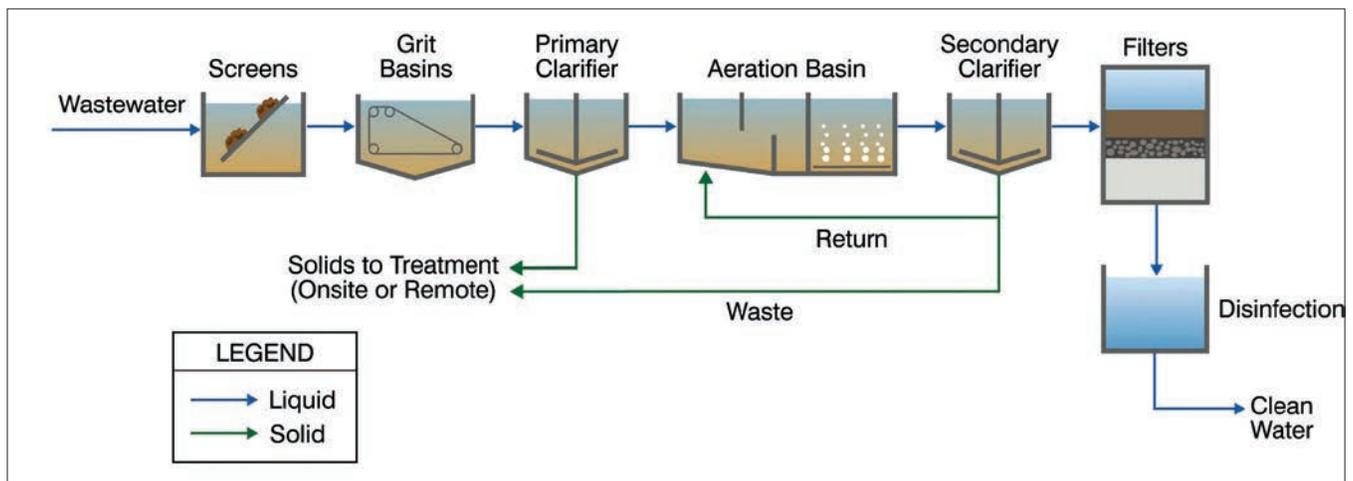
Figure 3: The current system of activated sludge plants [Available from <http://www.oakharborcleanwater.org/proposed-future-treatment-facility-technologies>]
