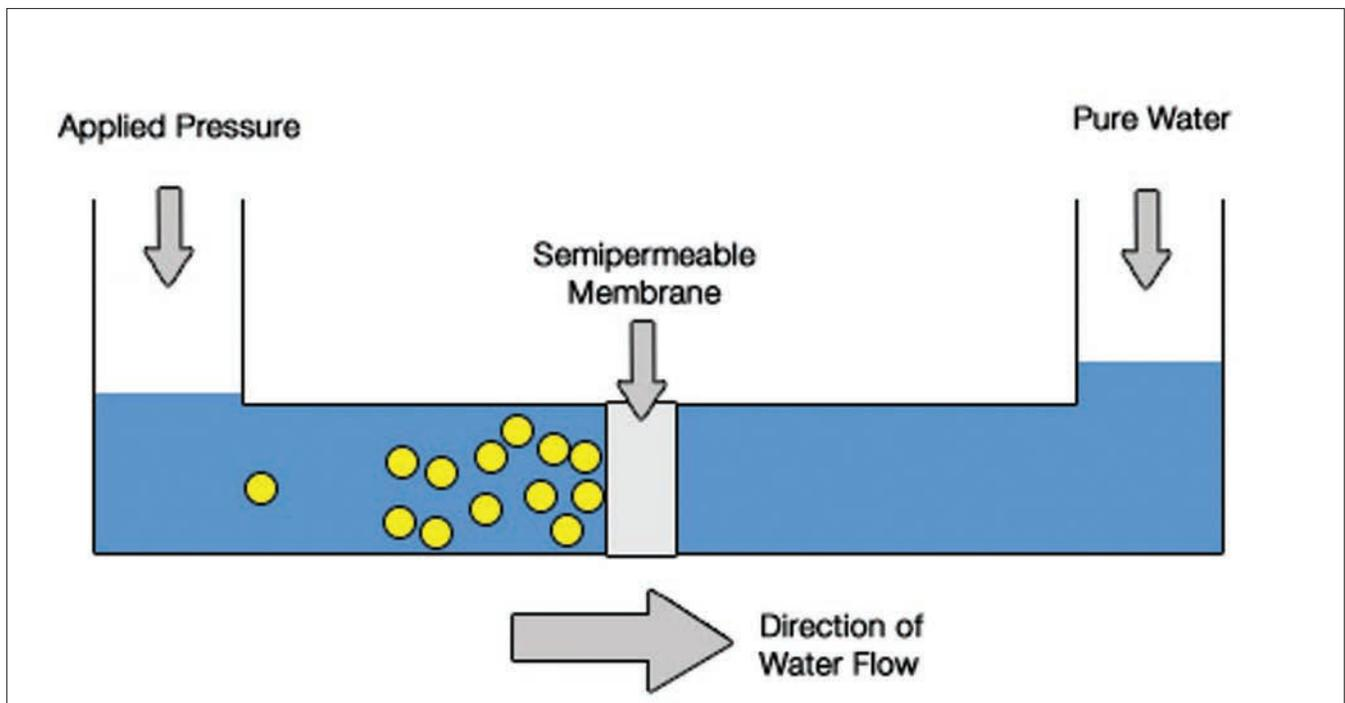
Figure 9: Image of reverse osmosis process [Available from [http://bmet.wikia.com/wiki/Reverse\\_Osmosis\\_Unit](http://bmet.wikia.com/wiki/Reverse_Osmosis_Unit)]
