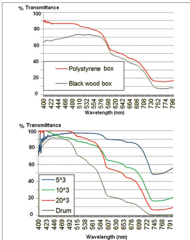
Figure 2: How transmittance varies across wavelengths for each dimension of the boxes (above) and cubes (below)
